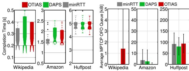
(a) 3G+WLAN, Completion time (b) 3G+WLAN, OFO queue
