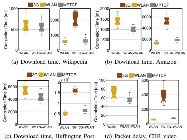
Figure 1. Download times for selected websites, and application packet delay for CBR video traffic, both over MPTCP in **WLAN+WLAN** (left of each pair) and **3G+WLAN** (right of each pair) (CORE emulation, with background traffic, see III-1). MPTCP with heterogeneous paths (**3G+WLAN**) underperforms single-path TCP on the best (WLAN) path.
