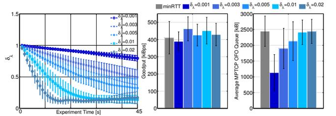
Figure 7. 3G+WLAN and BLEST's  $\lambda$  parameter influence on bulk traffic with varying  $\delta_\lambda=0.001, 0.003, 0.005, 0.01, \text{ and } 0.02$ ; compared against minRTT.
