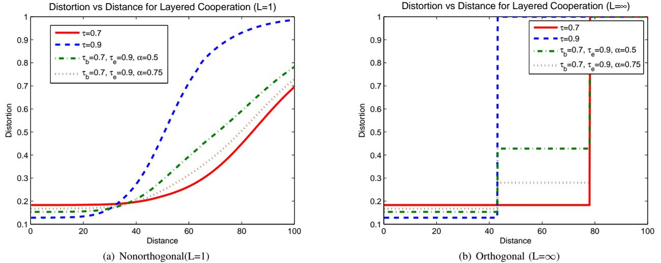
Fig. 3. Sequential Layered Cooperative Multicast: Comparison of end-to-end distortion for orthogonal and nonorthogonal relay transmissions ( $P_s = 10, \tilde{P}_r = 1, d_0 = 1, N_b = 5, N_e = 5, b = 8$ )
