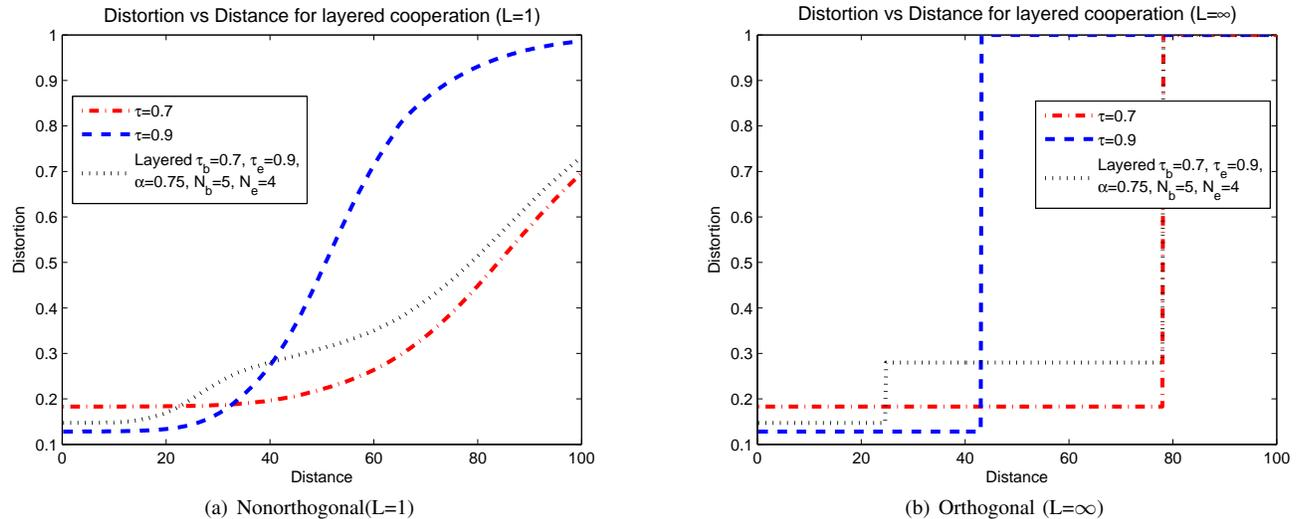
Fig. 4. Comparison of distortion for layered cooperation with different number of hops at base and enhancement layer ( $P_s = 10, \tilde{P}_r = 1, d_0 = 1, N_b = 5, N_e = 4, b = 8$ )
