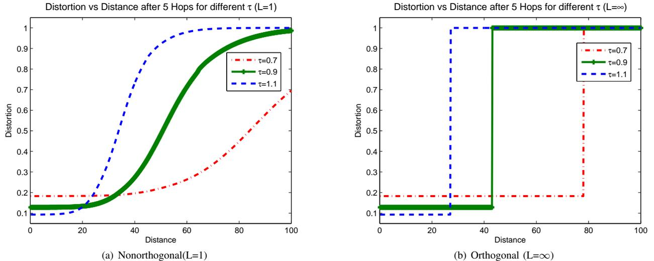
Fig. 1. Single Layer Cooperative Multicast: Comparison of end-to-end distortion for orthogonal and nonorthogonal relay transmission for different  $\tau$ 's ( $P_s = 10, \bar{P}_r = 1, d_0 = 1, N = 5, b = 8$ )
