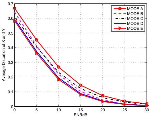
Fig. 6. Average distortion with  $\rho = 0.9$ ,  $SNR_x = SNR_y = SNR_{xy} = SNR$
