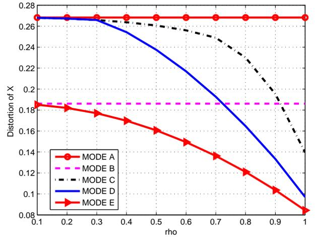
Fig. 7.  $D_x$  versus  $\rho$  with  $SNR_x = SNR_y = 10dB$ ,  $SNR_{xy} = 40dB$
